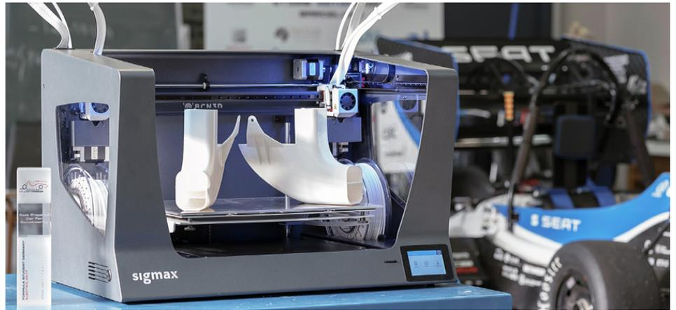
[Tecalum Industrial](#) also uses the Duplication mode for their benefit when [3D printing their customized clamps, toolings, jigs and fixtures](#). *"We benefit greatly from IDEX technology, as most of the time we need 2 or 4 pieces of the same clamps, so with the independent dual extruder system we are able to reduce production time in half"* confirms Marc Linares, Production Engineer at Tecalum.
