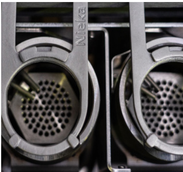
The crucible clips hold the sample in place while it's heated.
