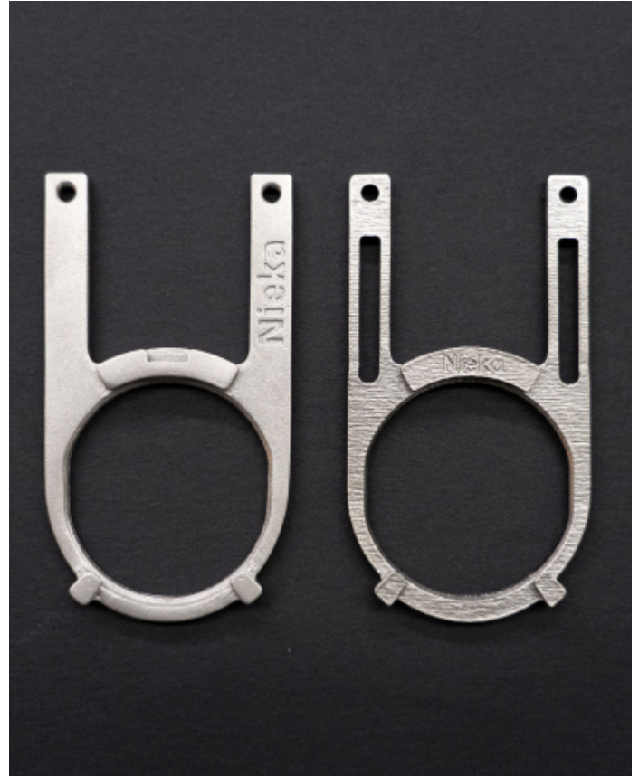
Markforged 3D printed crucible clip on the left, DMLS 3D printed crucible clip on the right.
