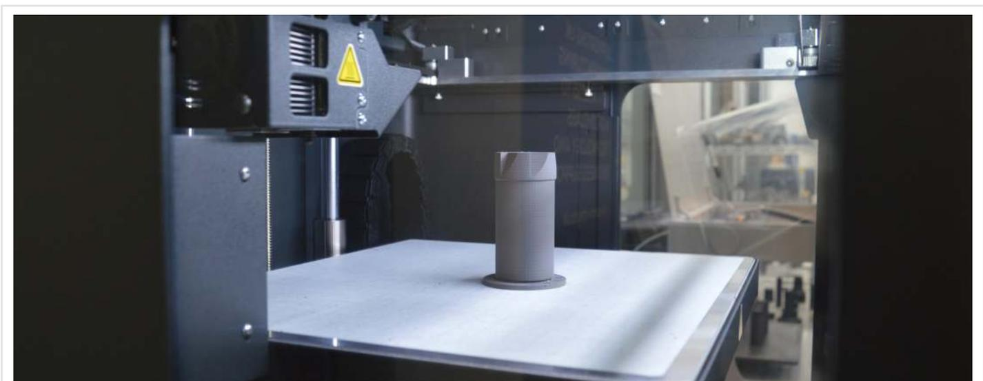
The engineers at Guhring UK have been able to rapidly prototype cutting tools in composite materials before printing them in metal.
