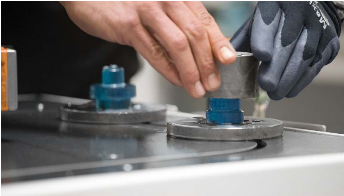
Each working stage in the automated lathe requires a custom jig. The jigs are attached to the conveyor belt using shuttles.
