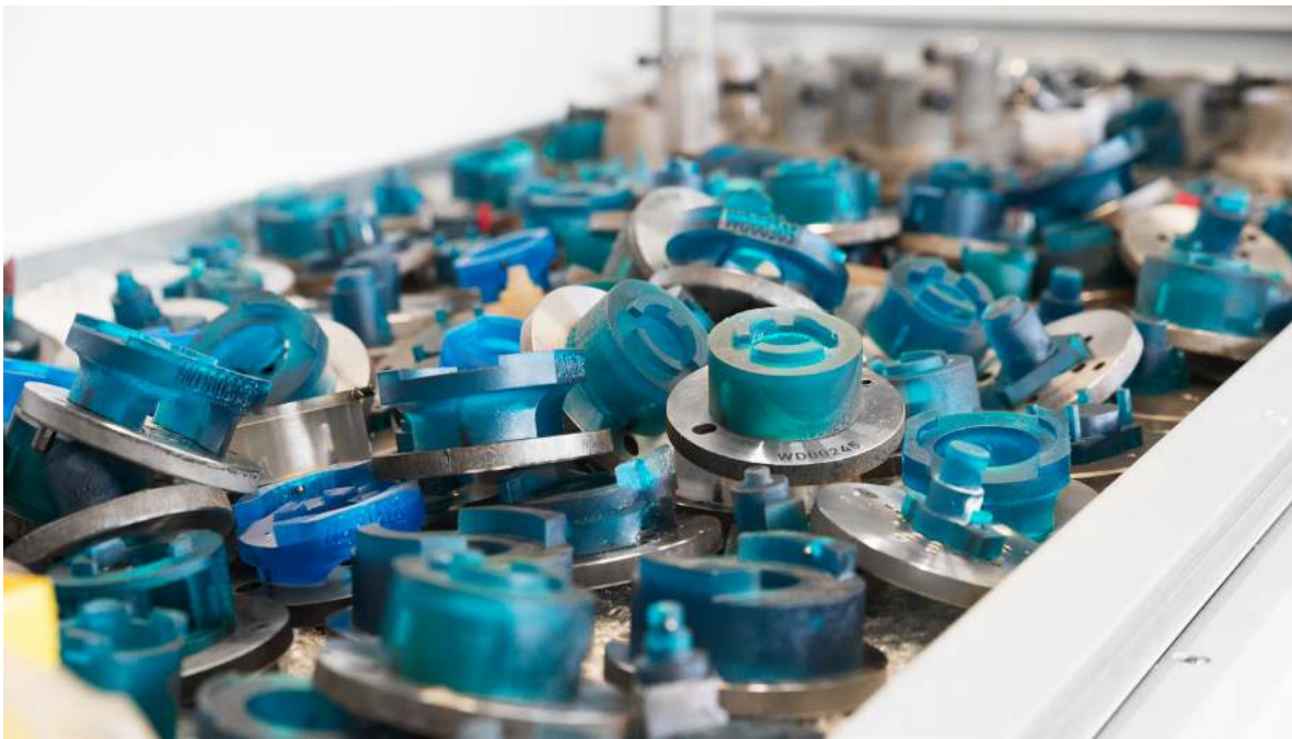
Each jig is printed with a unique identifier on its side.
