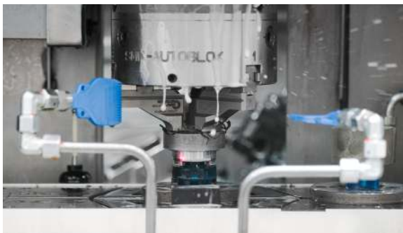
A machine picks up the parts from the first jig, and places it on the second jig once the machining process is complete.
