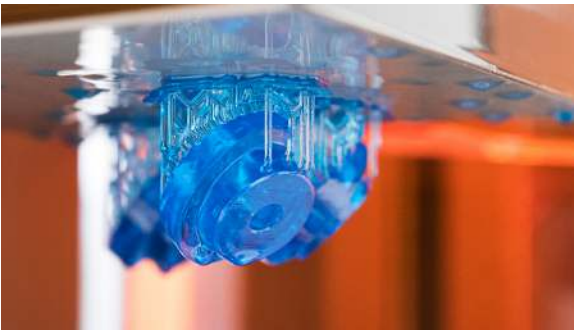
Jigs are 3D printed in batches using Formlabs Tough Resin.
