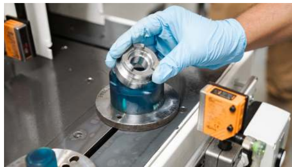
The finished parts are manually removed and cleaned of metal chips.
