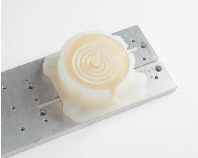
A part properly seated in a pocket jig printed in Formlabs Durable Resin.
