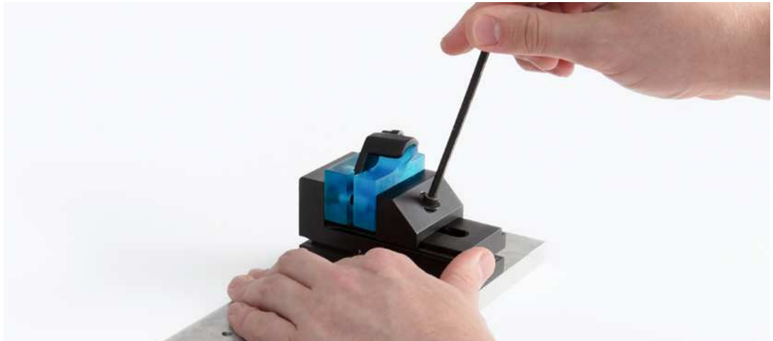
A part being clamped between soft jaw inserts, printed in Formlabs Tough Resin.
