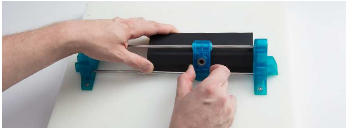
The drill jig slides smoothly across the steel rails by using Formlabs Durable Resin bushings pressed into the Tough Resin guide.
