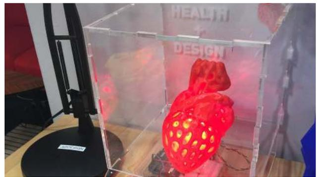
A 3D printed heart model wired with Neopixels and connected to an Arduino powered heart rate monitor to create a heart rate visualizer. Created by: Dr. Robert Pugliese
