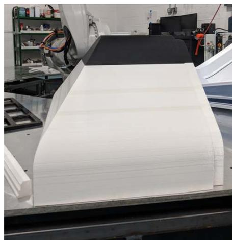
Another large mold, about 30 inches cubed this time, is a shroud mold made in two pieces for the Verizon digital kiosk. With 3D printing, the Boyce team discovered, a large, dense part becomes extremely durable – ideal for thermoforming. The team saved time and money again making this large mold from 3D printed plastic filament ahead of creating the final with traditional methods from aluminum.
