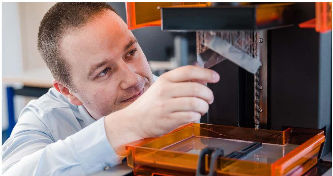
*Riegler's development department uses 3D printing to create prototypes for complex system components. Here, a cartridge cover is 3D printed using Formlabs Grey Resin at 25 micron resolution*
